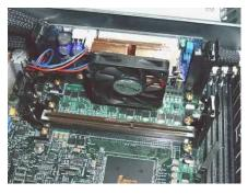
Inserting the first PL-P3/SMP into the processor slot.
